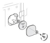
2 Insert a new backup battery (CR2032) with the + symbol on the battery facing outside.
